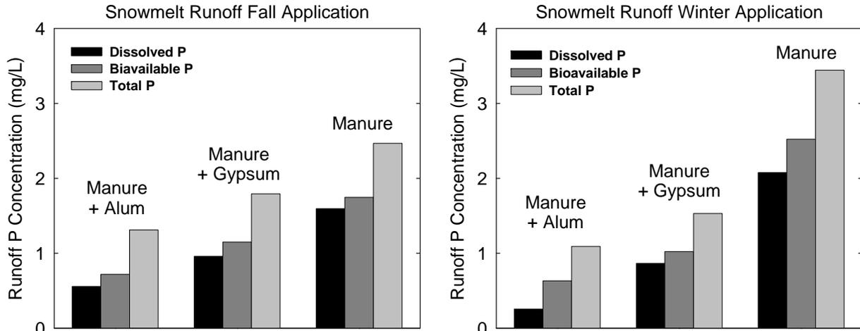
Fig. 4. Snowmelt runoff P concentration after applying poultry manure untreated or treated with alum or gypsum at 100 lb  $P_2O_5$ /acre in the fall without incorporation into the soil or in winter to snow-covered ground (averages of three years).
