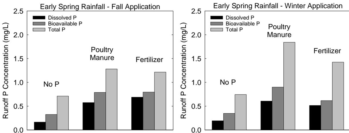
Fig. 5. Phosphorus concentration in spring runoff for plots where snowmelt runoff was collected and untreated poultry manure had been applied at 100 lb  $P_2O_5$ /acre in the fall without incorporation into the soil or in winter to snow-covered ground (averages of three years).
