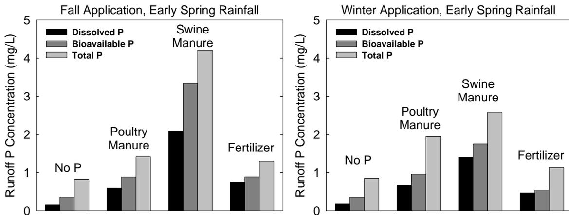
Fig. 9. Phosphorus concentration in early spring runoff for plots where snowmelt runoff was collected and no P, fertilizer, poultry manure, or swine manure had been applied at 100 lb  $P_2O_5$ /acre in the fall without incorporation into the soil or in winter to snow-covered ground (averages of two years).
