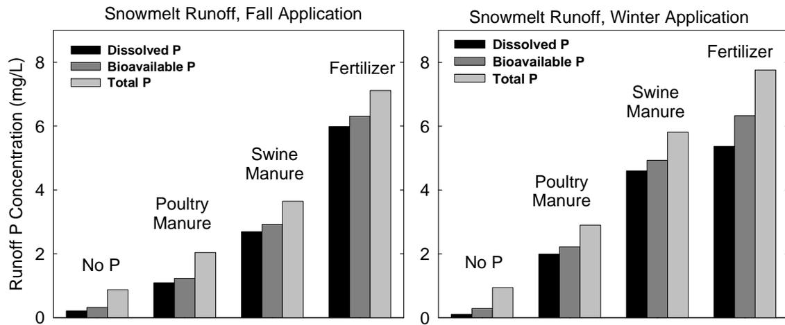
Fig. 8. Snowmelt runoff P concentration after applying fertilizer, poultry manure, or swine manure at 100 lb  $P_2O_5$ /acre in the fall without incorporation into the soil or in winter to snow-covered ground (averages of two years).
