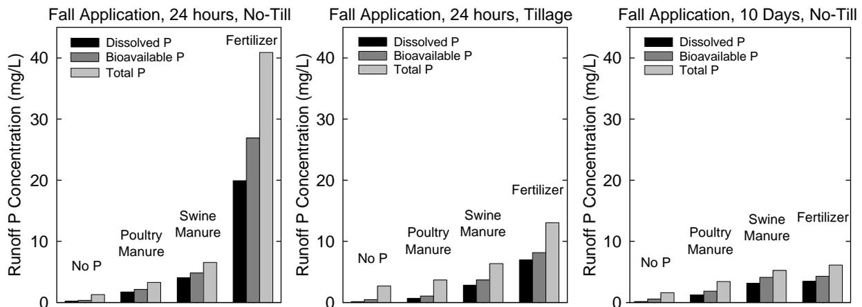
Fig. 7. Runoff P concentration within 24 hours of applying fertilizer, poultry manure, or liquid swine manure at 100 lb  $P_2O_5$ /acre in the fall with or without incorporation into the soil and also after 10 days of application without incorporation (averages of two years).
