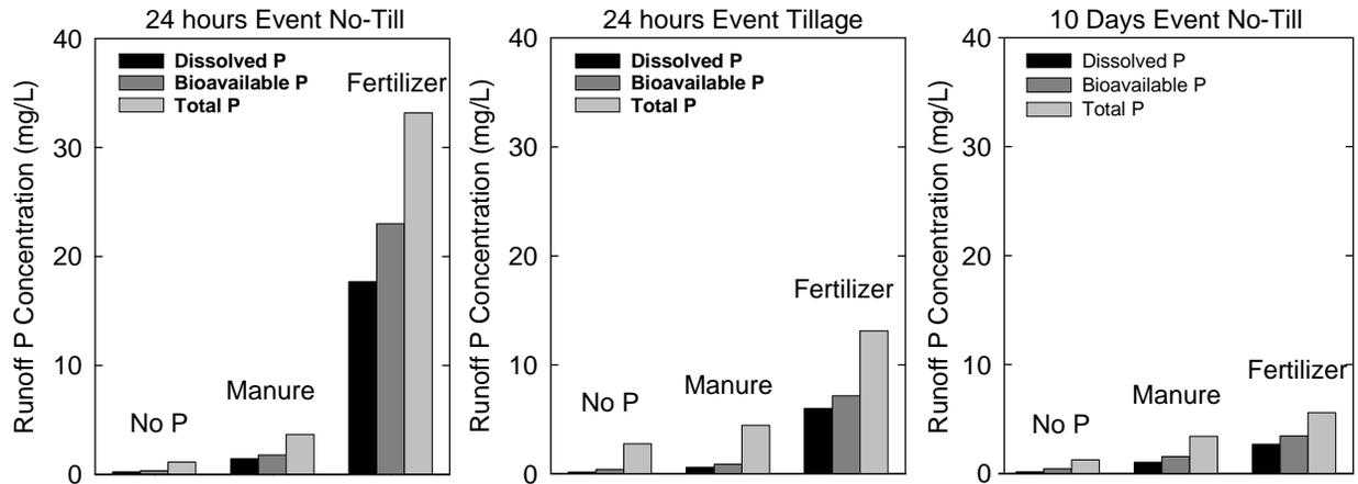
Fig. 1. Runoff P concentration within 24 hours of applying fertilizer (DAP) or poultry manure at 100 lb  $P_2O_5$ /acre in the fall with or without incorporation into the soil and also after 10 days of application without incorporation (averages of three years).
