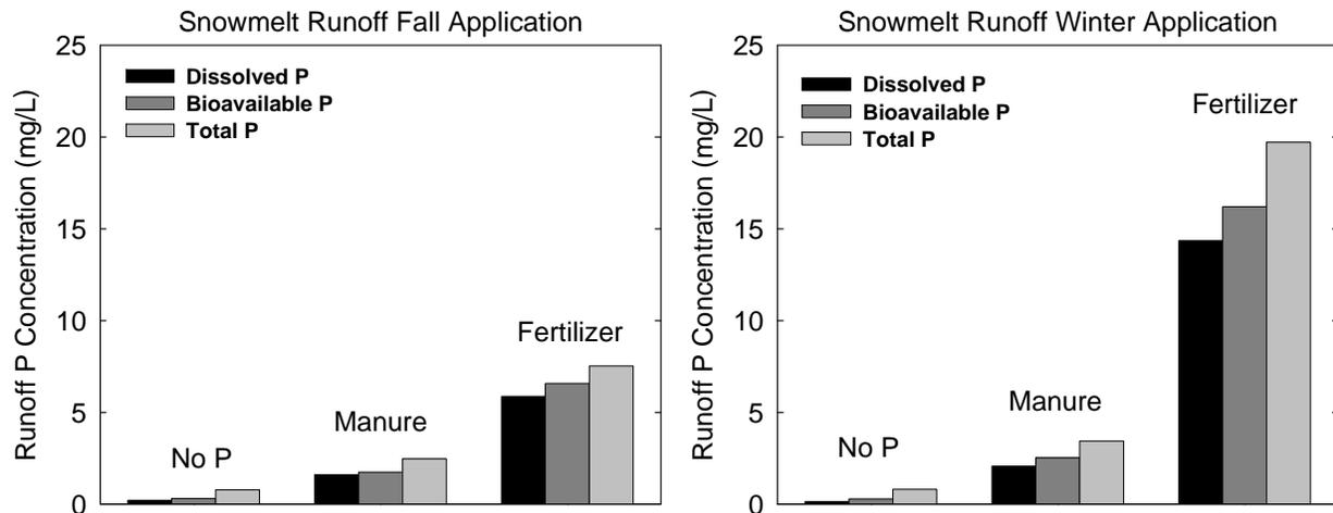
Fig. 3. Snowmelt runoff P concentration after applying fertilizer or poultry manure at 100 lb  $P_2O_5$ /acre in the fall without incorporation into the soil or in winter to snow-covered ground (averages of three years).
