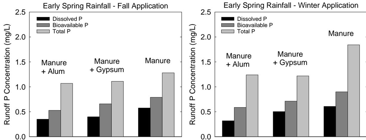
Fig. 6. Phosphorus concentrations in early spring runoff for plots where snowmelt was collected and poultry manure untreated or treated with alum or gypsum had been applied at 100 lb  $P_2O_5$ /acre in the fall without incorporation into the soil or in winter to snow-covered ground (averages of three years).
