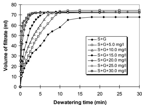
Fig. 2 Effect of polymer dosage on dewatering behaviour of 60% DS gypsum pre-added sludge (Conditioned sludge was poured into the piston chamber up to the depth of 2 cm. Applied pressure is 5.0 bar. In the legend, S refers to sludge, G represents gypsum and the values show the polymer dosage)
