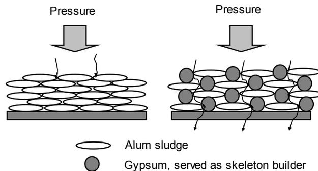
Fig. 5 Conceptual description of the role of gypsum as skeleton builder in sludge dewatering (Lai and Liu, 2004)
