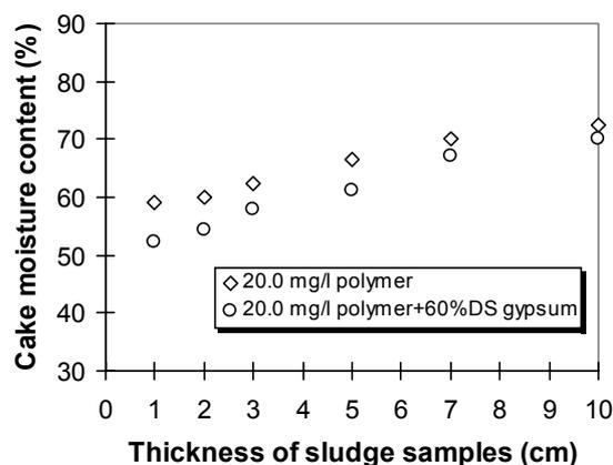
Fig. 4 Effects of thickness of sludge samples on cake equilibrium moisture content with and without gypsum addition (Applied pressure is 5.0 bar)
