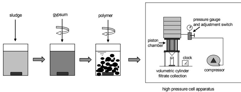
Fig. 1 Schematic illustration of experimental procedure
