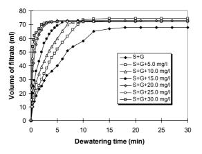
Fig. 2 Effect of polymer dosage on dewatering behaviour of 60% DS gypsum pre-added sludge (Conditioned sludge was poured into the piston chamber up to the depth of 2 cm. Applied pressure is 5.0 bar. In the legend, S refers to sludge, G represents gypsum and the values show the polymer dosage)
