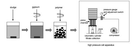
Fig. 1 Schematic illustration of experimental procedure
