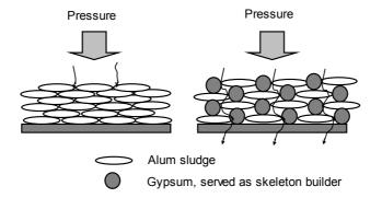
Fig. 5 Conceptual description of the role of gypsum as skeleton builder in sludge dewatering (Lai and Liu, 2004)
